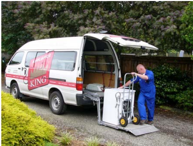
Figure 9.8.1 – Using a Lifting Platform
